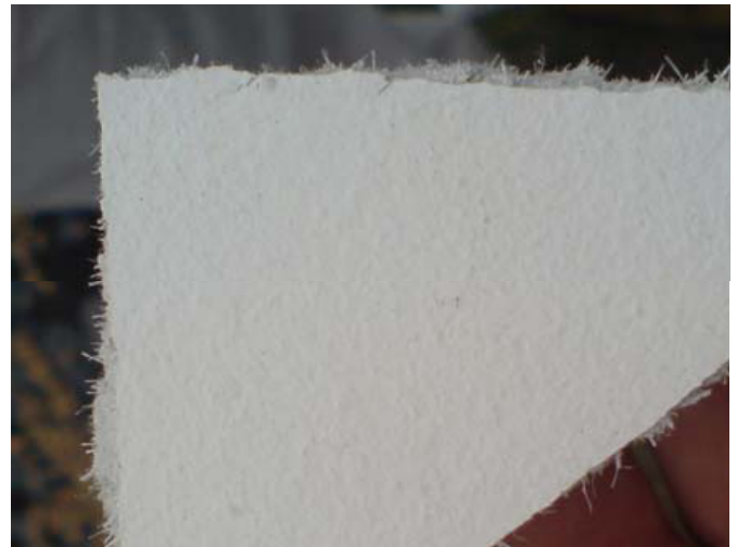
Photograph 2: Low density asbestos fibre board
